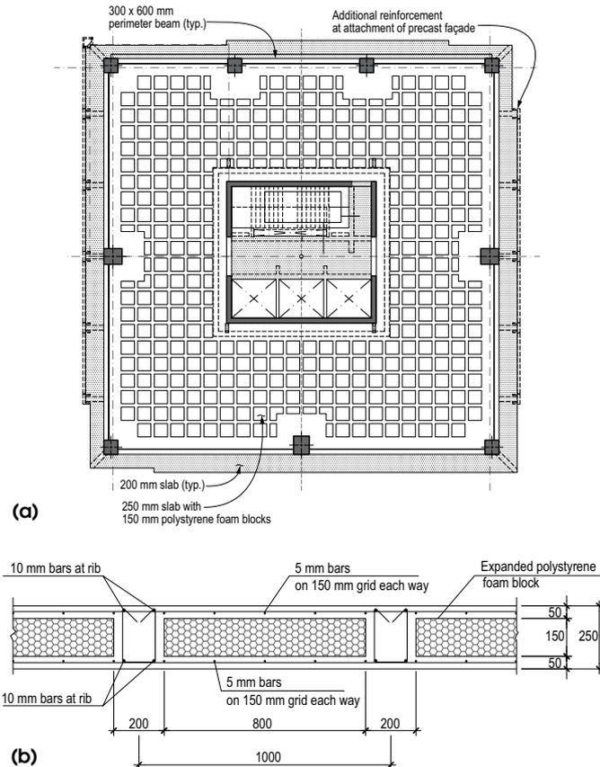
**Fig. 4: Structural drawings for the two-way PT concrete slab: (a) plan view showing border beam and central core; and (b) cross section of ribbed slab**
