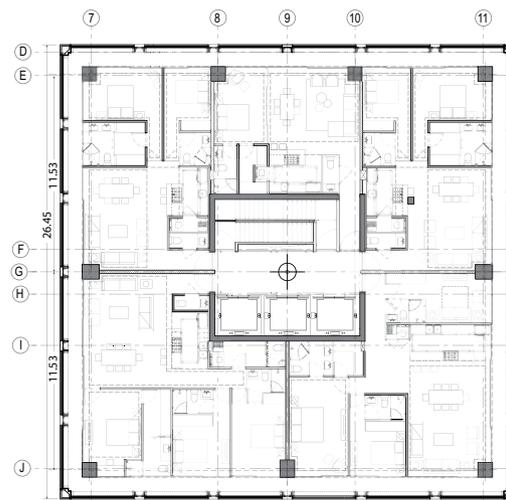
Fig. 2: Architectural floor plan of a typical residential level for Santa Fe II, showing central core, nine perimeter columns, and façade elements. The columns along the sides of the building were located to coincide with demising walls between individual apartments
