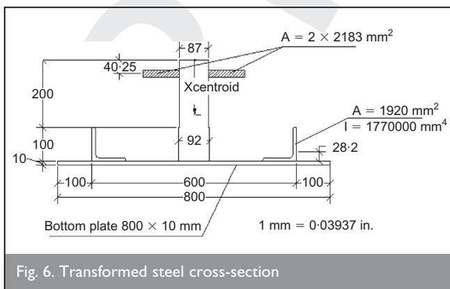
Fig. 6. Transformed steel cross-section
