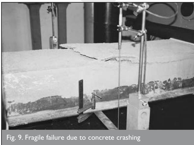
Fig. 9. Fragile failure due to concrete crushing
