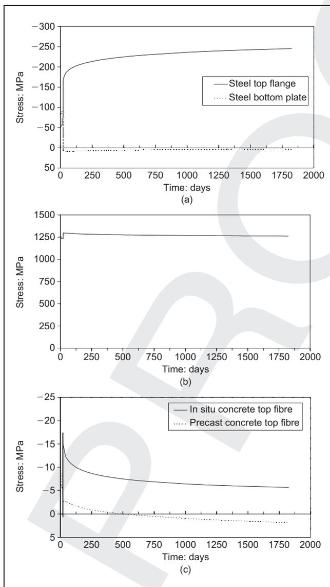
Fig. 14. Predicted redistribution of long-term stresses for service load (5 years): (a) steel shape; (b) prestressed steel lower layer; (c) concrete
