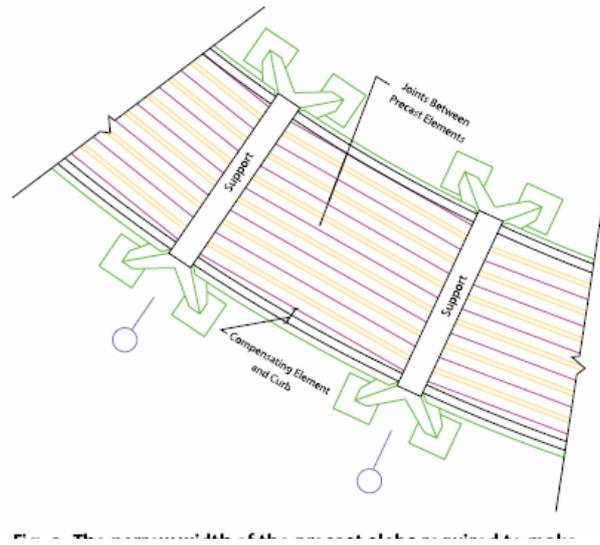
**Fig. 9: The narrow width of the precast slabs required to make them transportable also helps them work well with curved highway spans as shown for the JVC overpass in Mexico**
