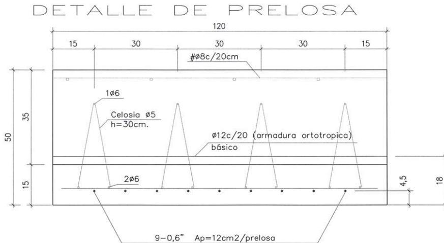
**Fig. 1: Typical complete section using the proposed system including a 150 mm prestressed precast slab, orthotropic positive reinforcement running perpendicular to the precast slab span, negative reinforcement in both directions at the top of the slab, and a 350 mm (13.8 in.) cast-in-place upper slab**
