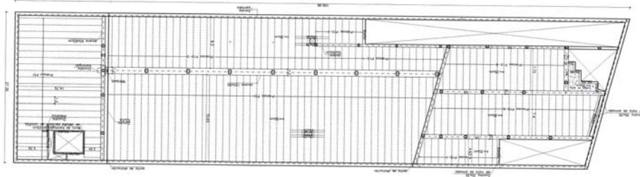
**Fig. 6: Structural floor plan showing the 17 x 55 m (56 x 180 ft) column-free area near the center of the building**
