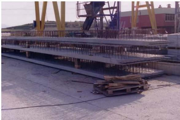
**Fig. 2: Prestressed precast slabs at ATEFOR casting yard in Barcelona-Spain**
