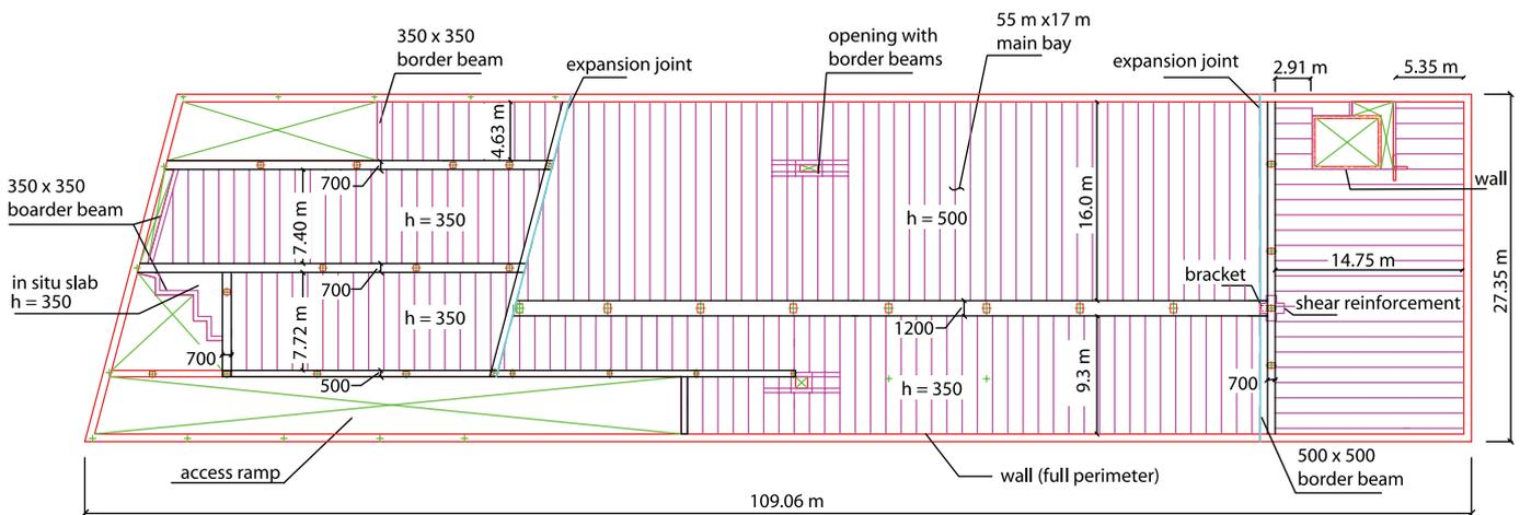
**Fig. 6: Structural floor plan showing the 17 x 55 m (56 x 180 ft) column-free area near the center of the building (all dimensions in millimeters unless noted otherwise; 1 in. = 25.4 mm; 1 ft = 0.3048 m)**
