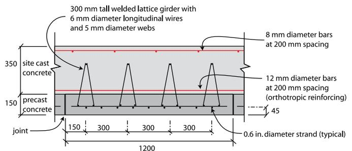
**Fig. 1:** This prestressed partially precast system includes a 150 mm (6 in.) prestressed precast slab, orthotropic positive reinforcement running perpendicular to the precast slab span, negative reinforcement in both directions at the top of the slab, and a 350 mm (13.8 in.) cast-in-place upper slab (All dimensions in millimeters; 1 in. = 25.4 mm)
