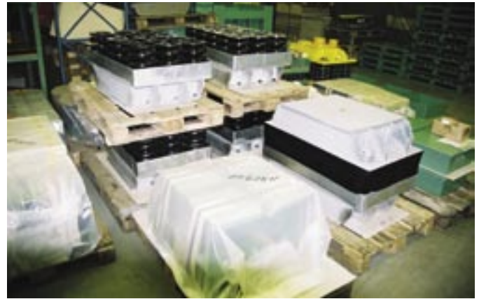
Fig. 3: Spring isolation units for the Sant Pau Hospital
